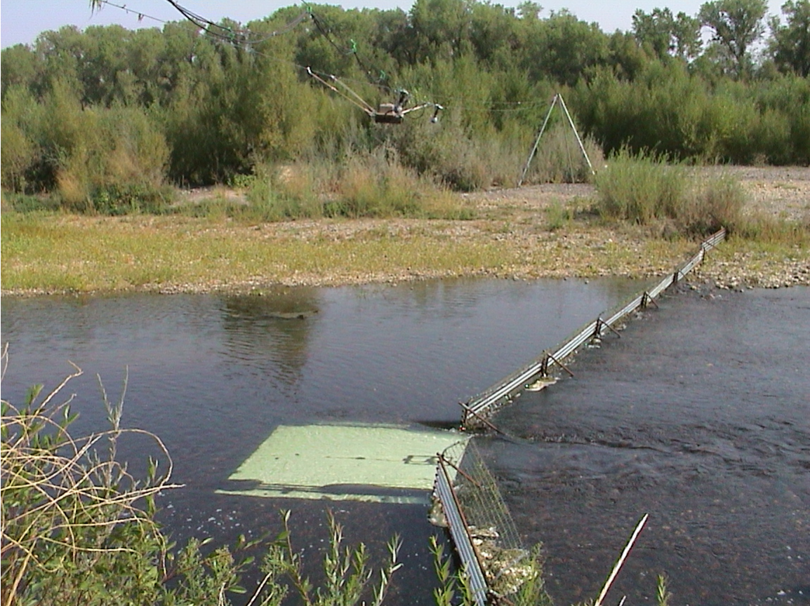
Figure 2. Video station camera box, lights, weir and passage opening with white plates visible. Camera is suspended from two overhead cables which are anchored to riparian trees and to a tall pipe tripod. Inside camera box is wiring junctions for electrical and video systems, and photo cell to turn lights on at dusk.
