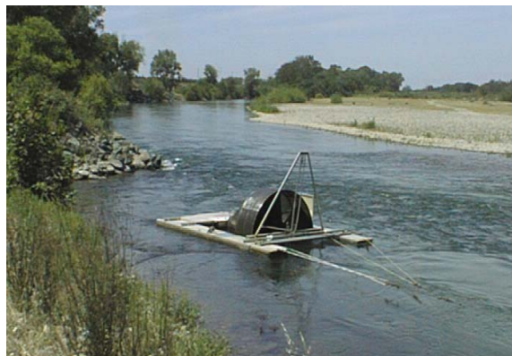
Figure 6. Rotary screw trap on Yuba River, near Marysville. Photo: K.True (USFWS)
