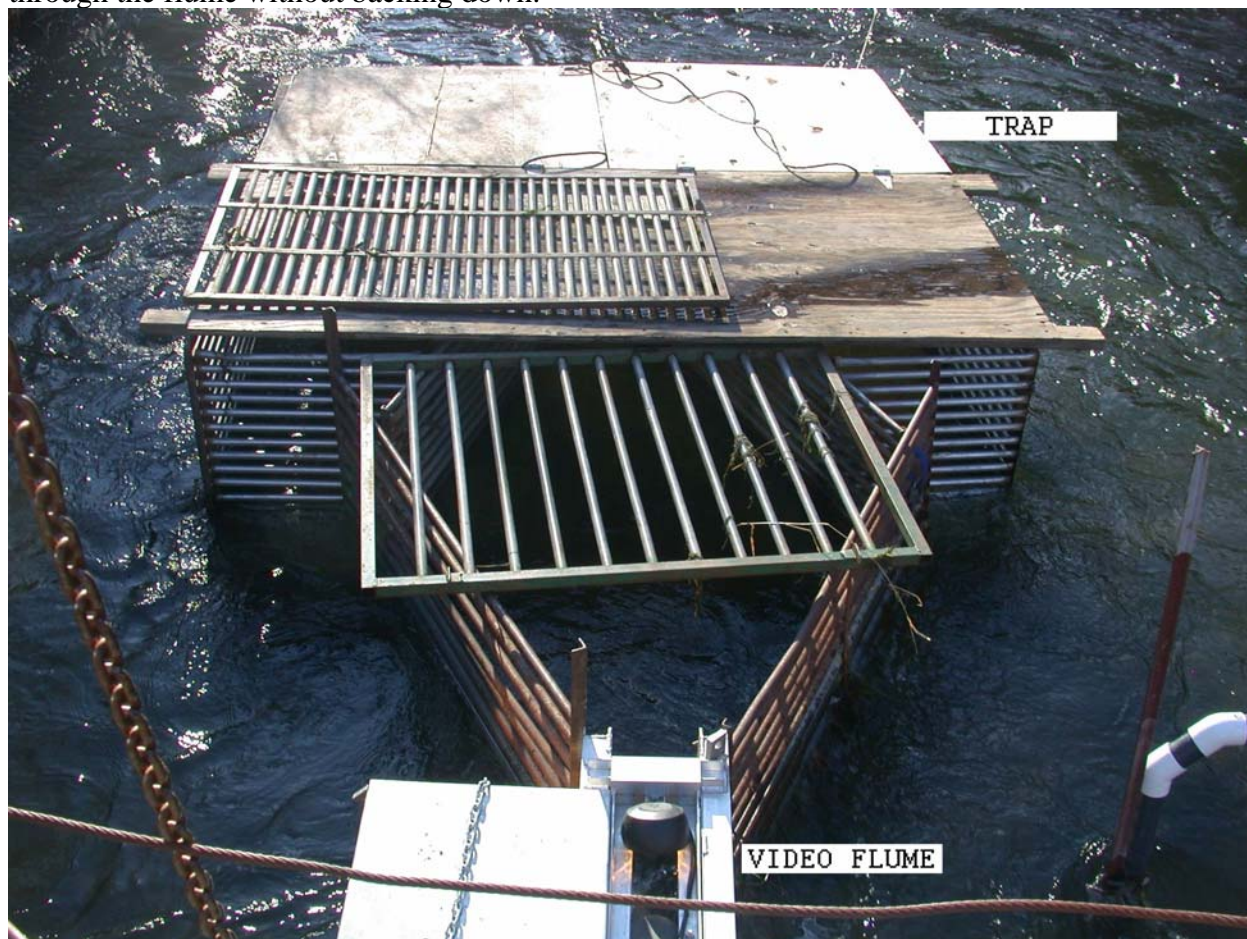
Figure 1. Coho trap attached to upstream end of video flume at SRFCE, 2007.
